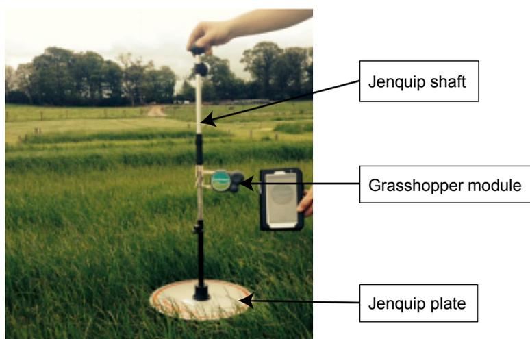
Figure 1. The Grasshopper module attached to the shaft of the Jenquip rising plate meter.
